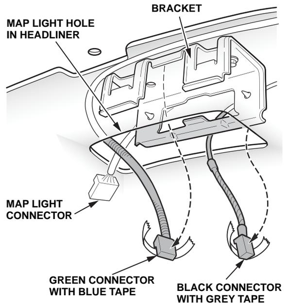
5. Remove the bracket bolt from the bracket.
